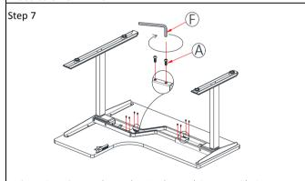
Tighten Crossbeams (part 4) using (part A) Screw M6\*10.
