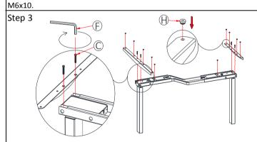
Attach the Side bracket (part 3) to the Crossbeam (part 4) using (part C) Screw M6x45. Rubber gasket (part H) into the hole on the Side bracket (part 3) and the Crossbeam (part 4).
