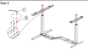
Attach Foot (part 1) to the Lifting leg (part 2) using (part B) Screw M6x16.
