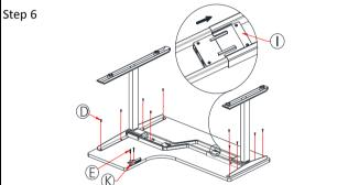
Adjust Crossbeams to the proper position to fit the desktop. Tighten the (part D) Screw ST6x14 to lock. Attach the Handset (part K) and Control box (part I) to the underside of the desktop using (part E) Wood screw ST4.2x16.
