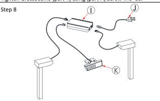
Connect the Lifting legs (part 2), Handset (part K), and the Power cable (part J) to the Control box (part I).
